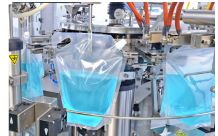
Filling of screenwash in stand-up pouches with corner spout
