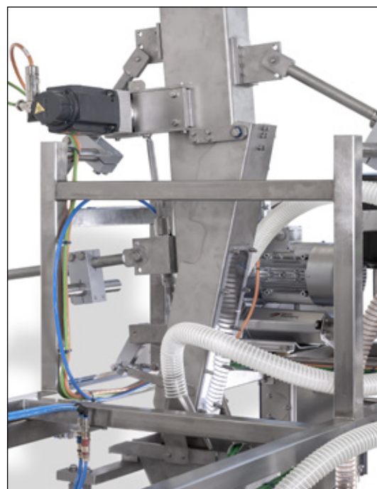
Servo motorized product flow control for large volume products
